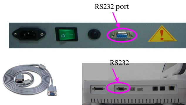
**NOTE:** The position of the RS232 port may be different on different treadmills.
