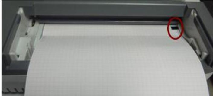
Reload the paper in the paper tray, close the recorder casing firmly. If the problem still exists, please contact the manufacturer or the local distributor for further disposal.
