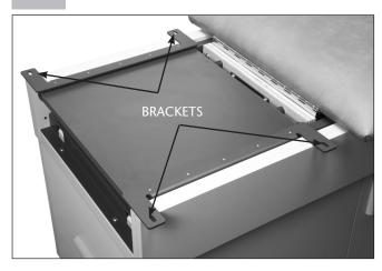
Secure the seat to the seat brackets using (4) four 1" hex head bolts and 3/4" washers.
