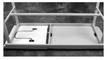
Use the hardware and tools provided to secure the legs into a locked position using the 1/4-20 x 1 ½" hex bolts and 1/4" locknuts, **DO NOT to tighten at this time.**
