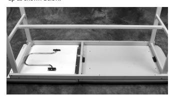
Use the hardware and tools provided 2 to secure the legs into a locked position using the 1/4-20 x 1 1/2" hex bolts and 1/4" locknuts. **DO NOT to tighten at this time.**
