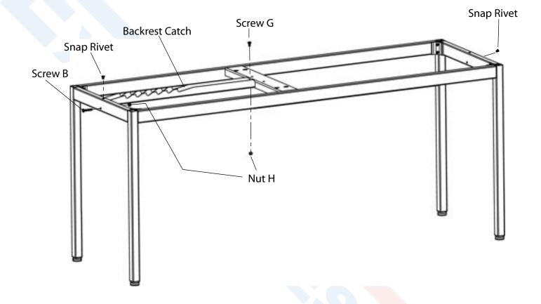
STEP A: Install Backrest Catch as shown in the drawing above. **CAUTION** The Backrest Catch needs to be positioned on top of the Tab shown in STEP 2.
