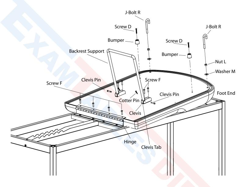
STEP A: Lay upholstered backrest on Foot End of frame as shown.
