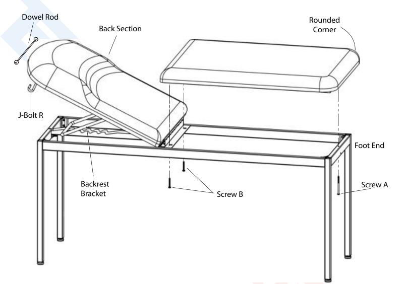
STEP A: Rotate Back Section until Backrest Bracket is engaged or top is horizontal on frame.
