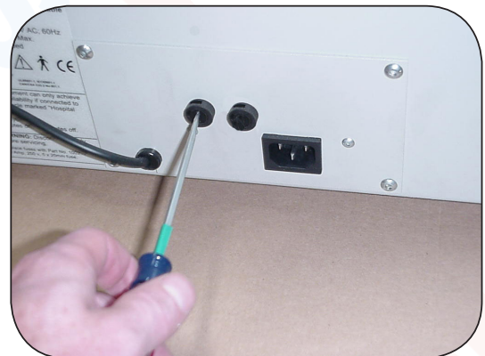
Figure 49. Tables with drawer warmer and no outlet use two 1A fuses.
