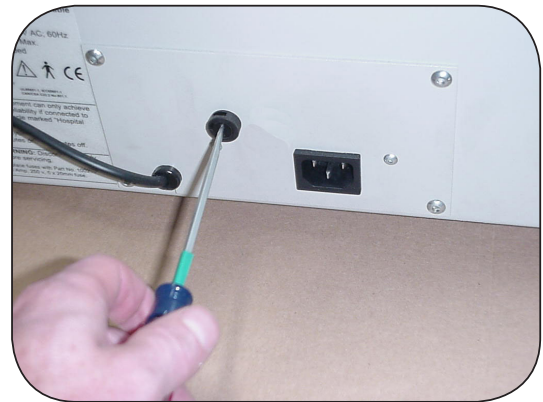
Figure 48. Tables with outlet and drawer warmer use a single 3A Fuse.
